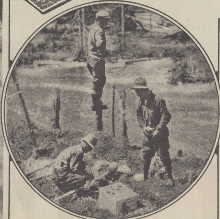
PREPARING A DYNAMITE CHARGE —Sticks of explosive tied to the end of a long pole, a detonator and fuse complete the equipment used to blast a log jam loose. Compression for the explosion is had by placing the dynamite in the water under the logs.
