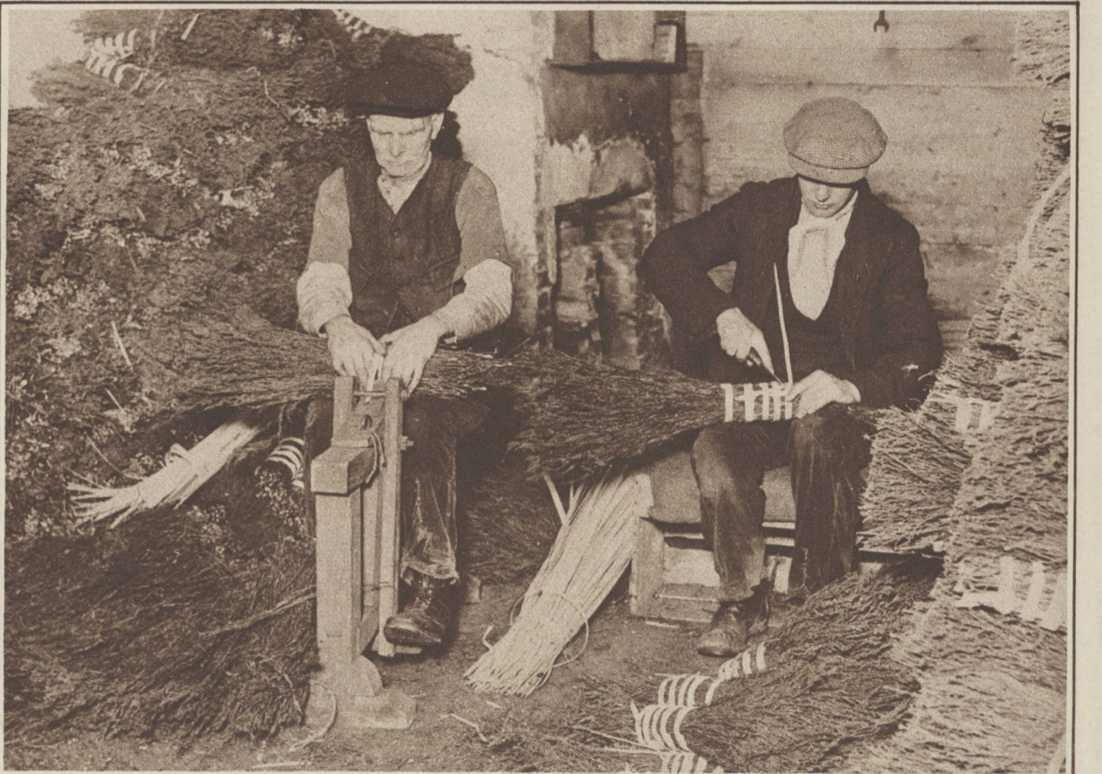
SIXTY-ONE YEARS OF BESOM MAKING—Joseph Bell, at the left, at the age of ten entered the trade of making besoms or brooms of heather and birch twigs bound with strips of ash, at his home at Winlaton, Durham, England. After sixty-one years he is still at it, and is seen here at his shop with his son. (Chicago Tribune Press Service photo.)
