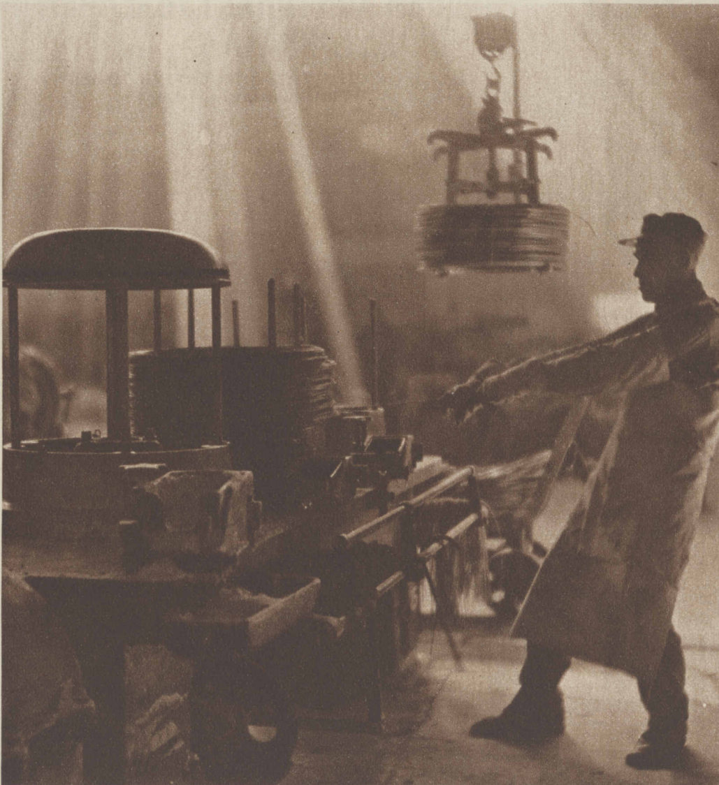
RIBBONS OF GOLD —Under slanting sunshine, man and machine pull fat steel rods through graduated holes, and the metamorphosis of steel wire is completed.
