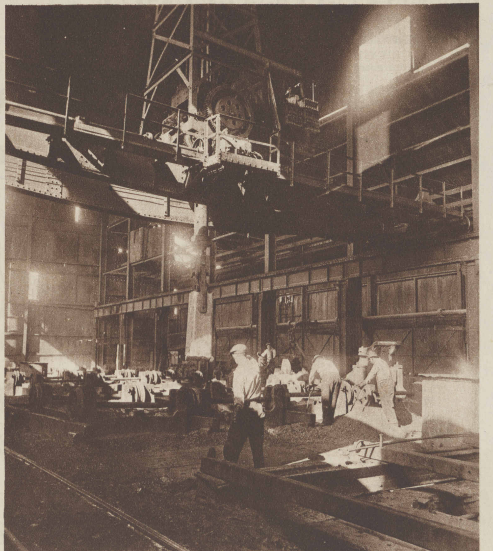
DAYTIME IN THE STEEL MILL —Sunshine pours down on workers at the "soaking pit," where ingots are reheated before rolling operations. (Hutchinson photos, from Colorado Fuel and Iron company.)
