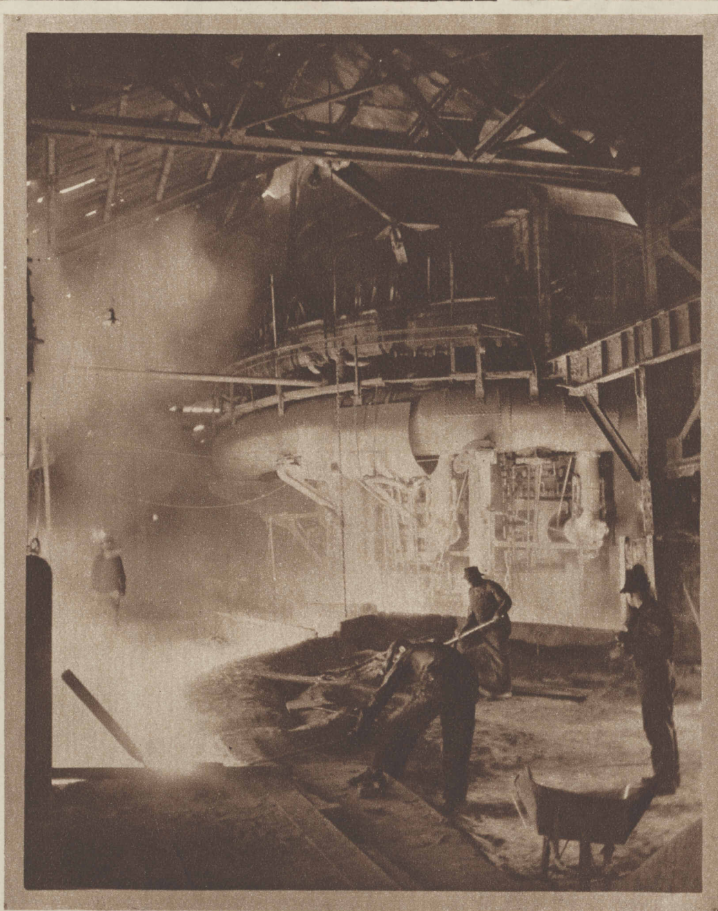
THE FLARES OF AN EERIE REALM —Flowing slowly down a bed of sand into submarine-shaped ladles, the stream of molten iron lights the steel mill with a fierce and unearthly glare.
