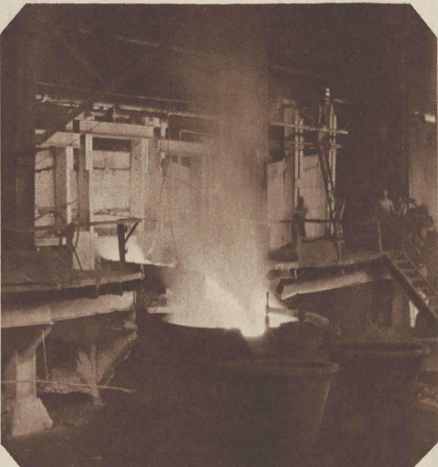
A RIVER OF MOLTEN METAL —The tapping operation, one of the most dramatic and spectacular moments of the steel worker's routine, has been completed, and the liquid steel flows into the gigantic pouring ladle, which has a capacity of many tons.
