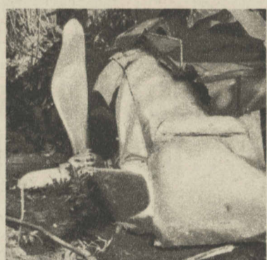
The left outboard engine of the strato-liner, lying a quarter of a mile from the main wreckage. Notice unfeathered propeller.
