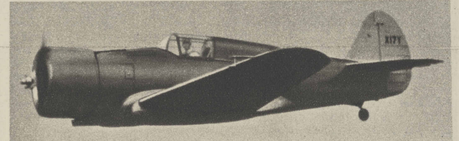
The American version of the single-seat fighter—Curtiss P-36. The engine is a twin-row Pratt & Whitney Wasp rated at 1,200 horsepower. The army air corps has ordered 210 of these planes.
