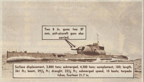
THE BIGGEST SUBMARINE IN THE WORLD is the French Surcouf, a diving corsair mounting the most powerful guns permitted by treaty. This nimble fighter submerges in two minutes. It is an experimental type, however, which France is not considered likely to repeat.
