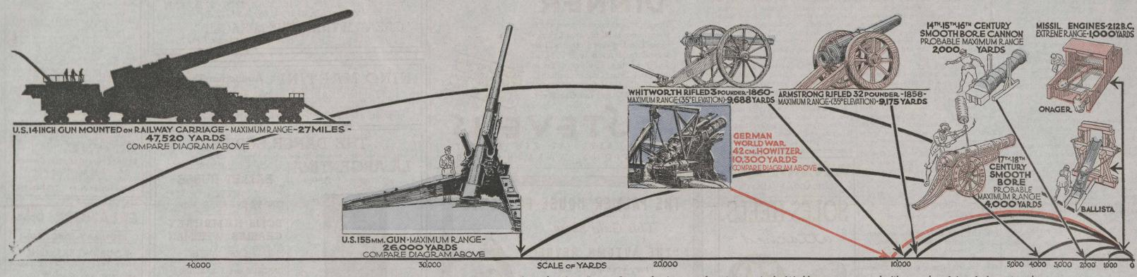
Examples of artillery typical of their times, and their respective ranges, from the ancient missil engines of 212 B. C. to the 42-centimeter German howitzers used at Antwerp in the World war, as compared with examples of America's most modern guns.
