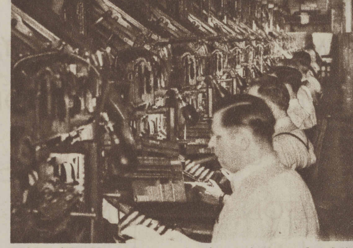
MORE THAN 100,000 words, the equivalent of a full-length novel, are contained in an average daily issue of the Tribune. Shown above are a few of the 72 linotype machines at which expert operators working under scientifically designed lighting equipment in an air-conditioned room convert this daily deluge of words into type.
