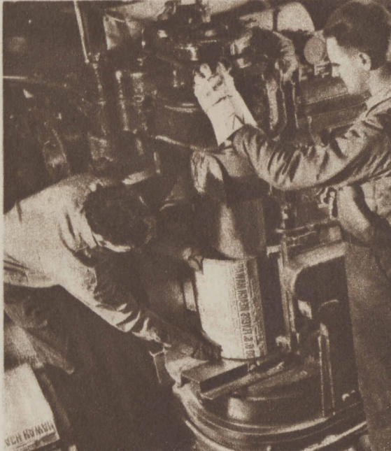
SEVEN AUTOMATIC autoplate machines like this cast from matrixes the curved 50-lb. metal stereotypes from which the Tribune is printed. Each plate is made in fifteen seconds. Over 800,000 stereotypes are cast each year.
