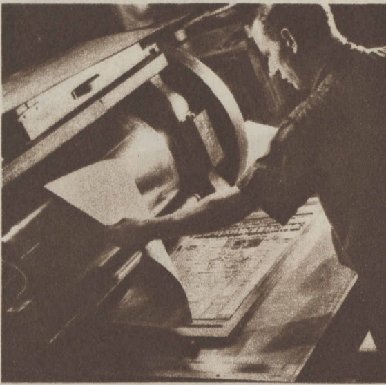
CONTINUOUS ADOPTION of better methods results in a better newspaper for readers and easier, safer tasks for workmen. In the picture above a matrix, after passing under a roller at a pressure of many tons, is being lifted from a form containing type for a Tribune page.
