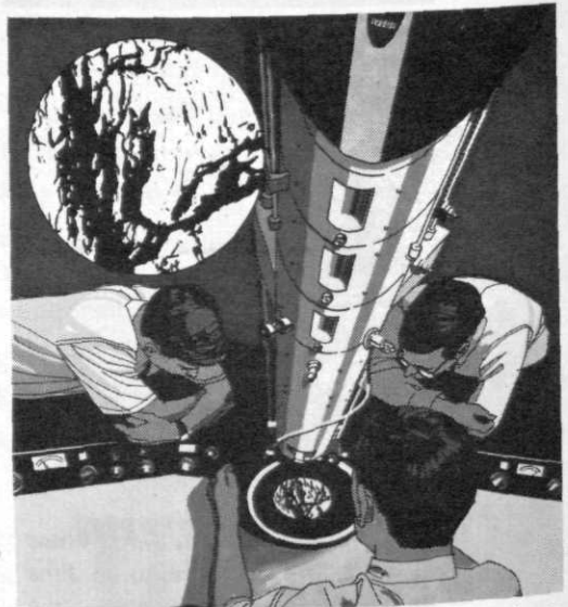
IH research engineers study fracture (see circle enlargement) of high strength steel in electron microscope. Scope has magnification potential of 5 million times.
