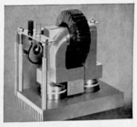
The new system employs the use of gallium arsenide, a semiconductor material which provides larger bandgaps and hence higher efficiencies and temperature capabilities. The tunnel diode inverter system has the advantage over previous designs in the following areas:
