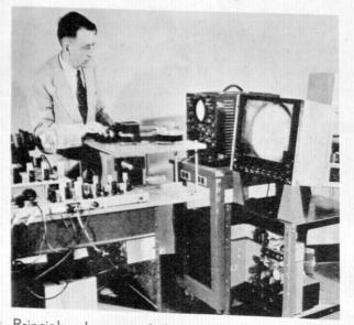
Principle elements of the sending terminal of the Ultrafax system.
