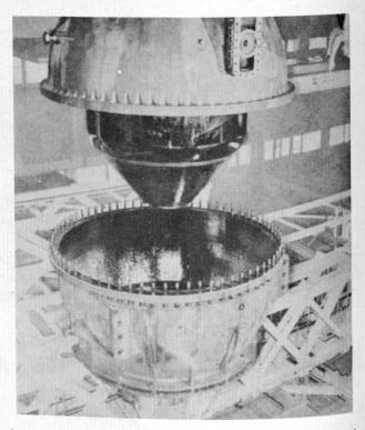
King-sized needle valve used to regulate water flow at the Bureau of Reclamation's Friant Dam in California.
