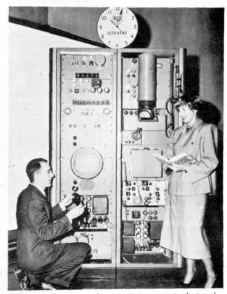
Apparatus used at the receiving terminal in the Ultrafax system.
