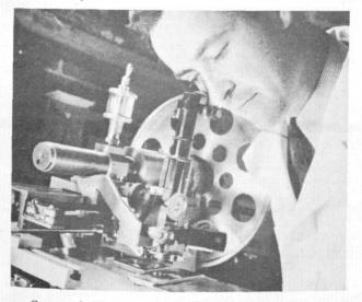
General Motors and Chrysler are cooperating in an effort to produce a set of accurately ruled geometric surface finish specifications which are to act as gauge blocks for surface finish measurement. All sets of the specimens will be replicas of one master set, so that complete uniformity will be assured.
