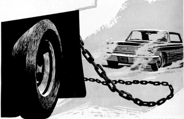
In chain-drag test, truck raises heavy dust clouds to check air filter efficiency.
