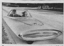
**Gyron**—dream car that drives itself. A gyroscope would stabilize this twowheeled vehicle of the future, which envisions automatic speed and steering control. A computer would let you "program" trips on a non-stop highway. For lasting beauty, trim areas would be coated with Nickel-Chrome plating, the bright, corrosion-resistant finish.
