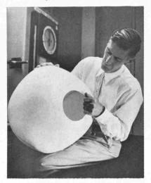
Once aloft and inflated, the object would soon rigidize and maintain its shape even though it was punctured by meteors, punished by temperature extremes, and exposed to ultraviolet radiation and other cosmic forces. These coatings are applied to the fabrics to impart a "rigidizing" capability and to form a film or barrier in the porous surface of the material so that it can be inflated when used in space structures.
