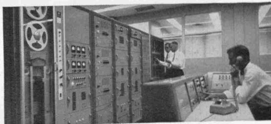
Representative of electronic aids functioning for P&WA engineers is this on-site data recording center which can provide automatically recorded and computed data simultaneously with the testing of an engine. This equipment is capable of recording 1,200 different values per second.
