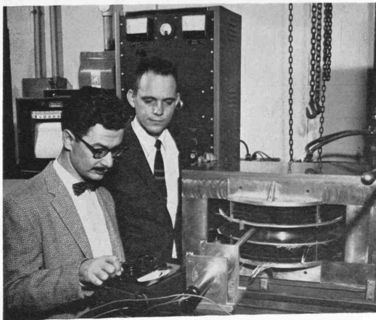
A close-up view of the model magnet and probe. By inserting probes between the magnet's pole faces, the magnetic field may be measured at various points. This data will show how the atomic particles will move in the completed cyclotron.
