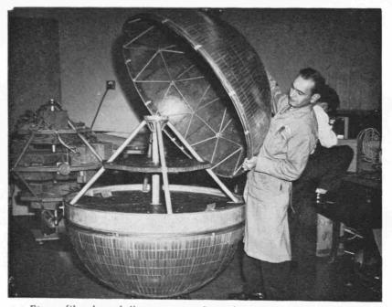
Epoxy fiberglass shells are mounted on dummy structure to check fit of parts. Wooden mock ups are used to determine exact location of the 38 "black boxes" making up the Courier payload.
