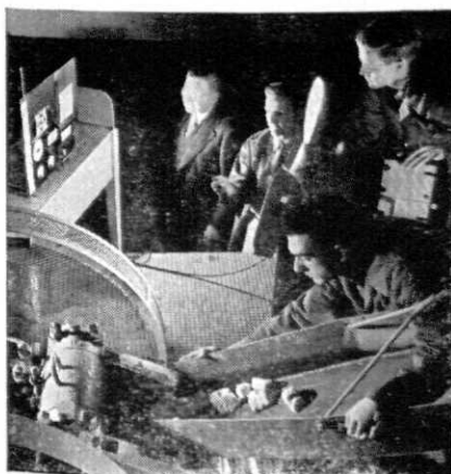
Studying power and capacity factors in ore crushing, in Allis-Chalmers' complete basic industries laboratory. Camera-recorded data will be applied to commercial mining operations.
