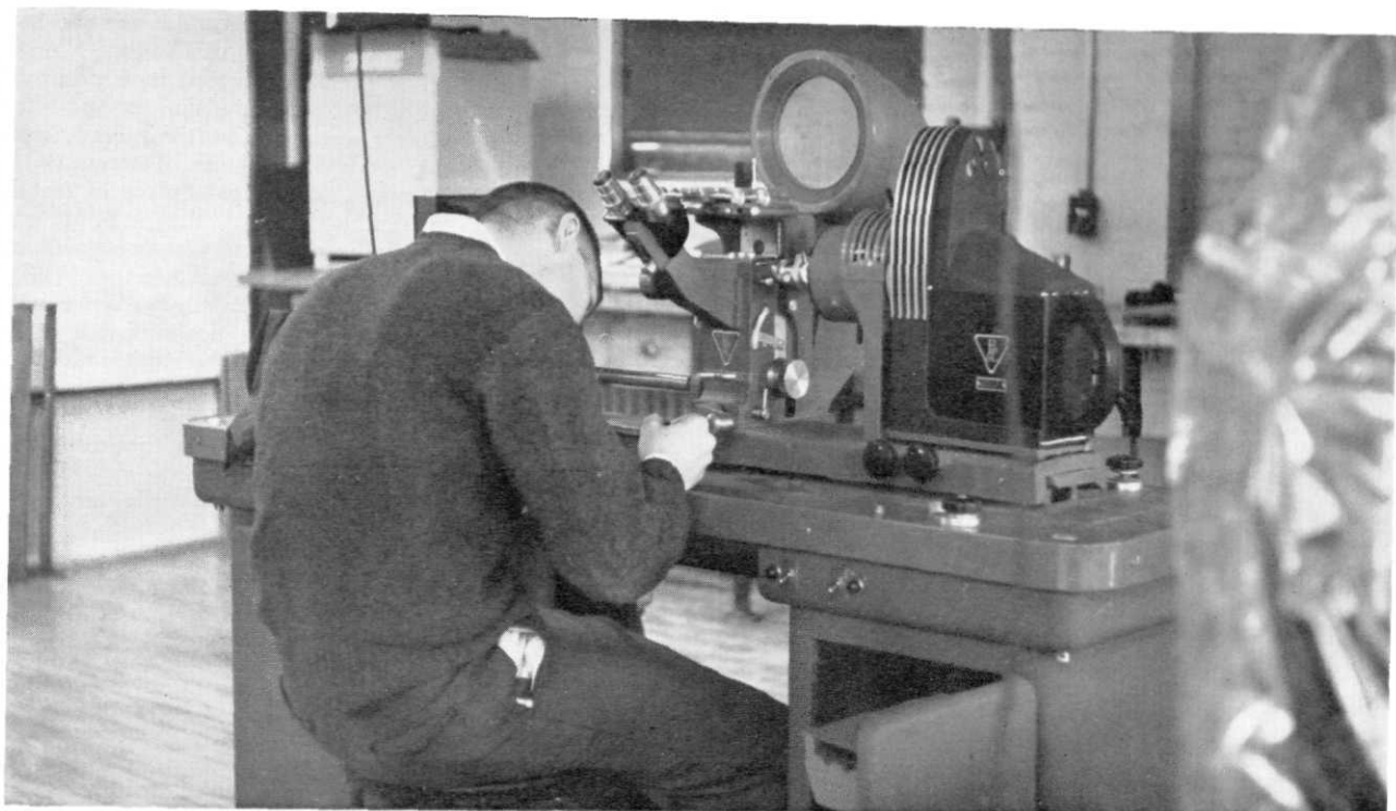
The microscope is one of the most powerful tools for studying metal structure. Dale Koch prepares an oil immersion objective lens for examining his sample at the highest resolution obtainable with a light microscope.
