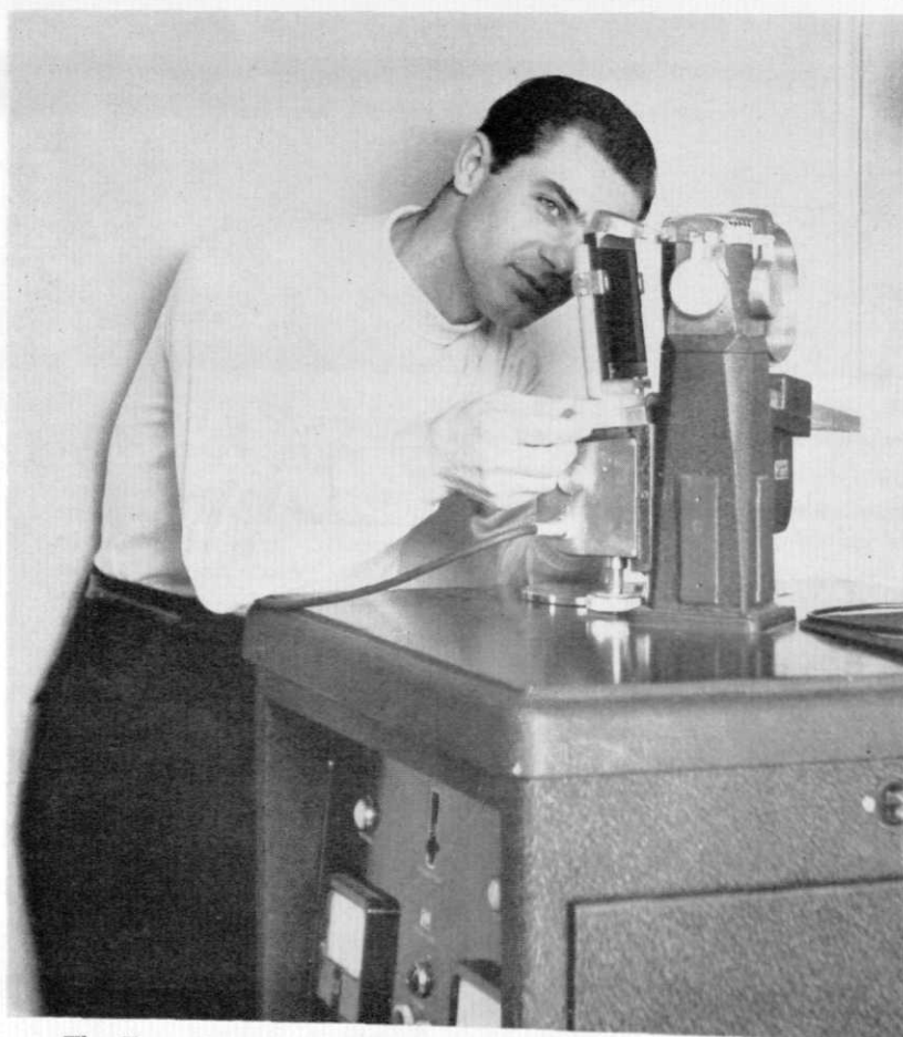
The X-ray is used for determining the ultimate atomic structure of the metals. Harry Richter lines up a flat plate camera for determining crystal orientation.
