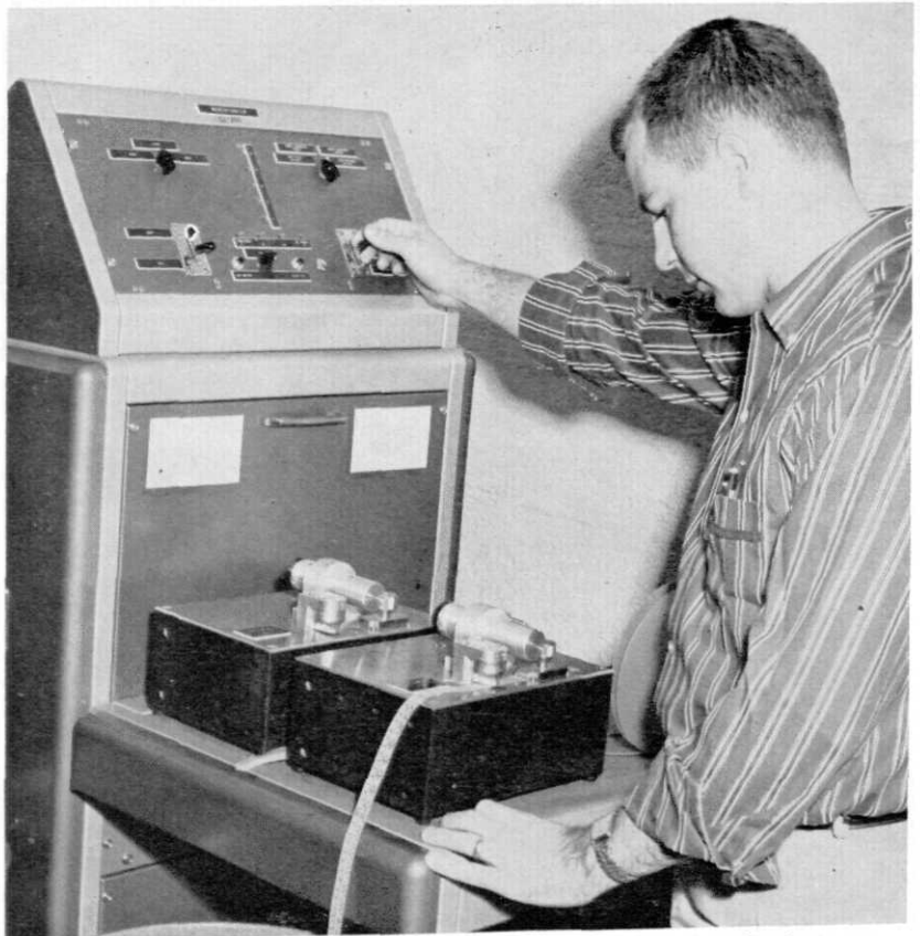
The perforator provides a means of copying or correcting programming tapes.
