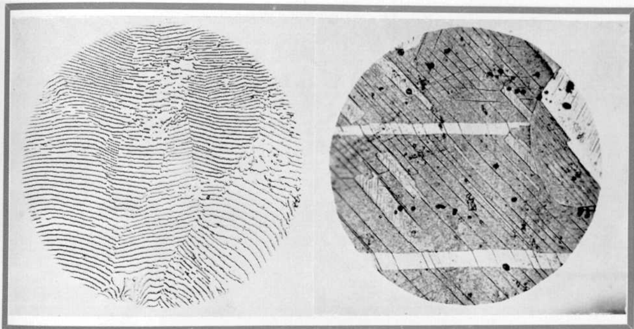
Slip Lines in Yellow Brass (Plastic deformation indicated by the parallel dark lines. Magnified 500 diameters.)
