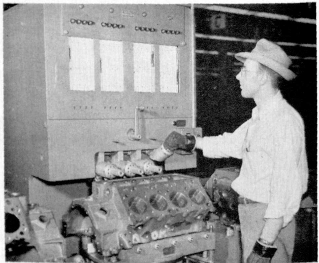
This multiple air gage is used to classify cylinder bores into one of 8 classifications by .00025 step. There is a metal stamping arrangement enabling the operator to stamp the bore size designation adjacent to each cylinder. In addition, during this sizing operation, the inspector can observe the taper and out-of-round characteristics of each bore by simultaneously measuring 4 points in each bore.
