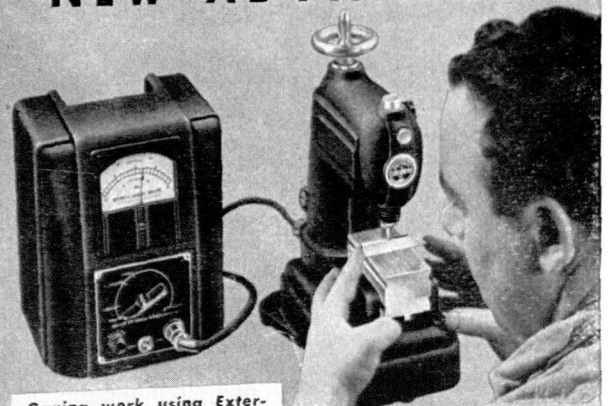
Gaging work using External Comparator No. 951 and Amplifier No. 950.
