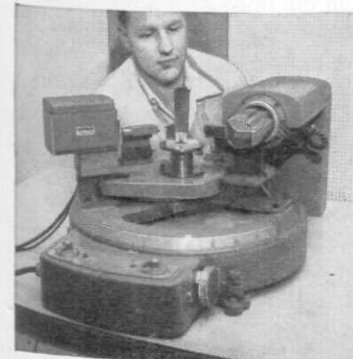
Engineer measures residual stress in a compressor blade non-destructively, using X-ray diffraction. Stress analysis plays important part in developing advanced aircraft engine designs.
