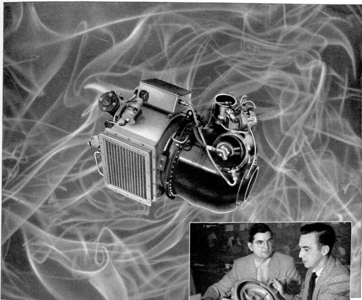
AiResearch two stage lightweight gas turbine compressor provides pneumatic power for aircraft main engine starting and serves as auxiliary power source for a variety of ground and in-flight services.
