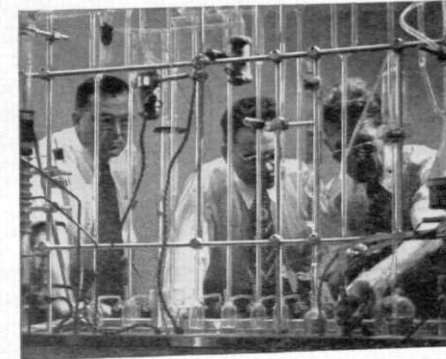
The important effects of gases on the properties of metals have been increasingly recognized. Pratt & Whitney chemists are shown setting up apparatus to determine gas content of materials such as titanium alloys.
