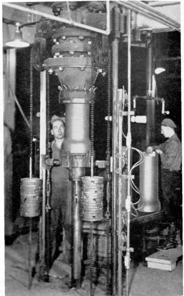
Fig. 2. Pulverized and mixed with water into a uniform, doughy mass, clay is die-pressed into pipe shape under tremendous pressure with either steam or hydraulic press.
