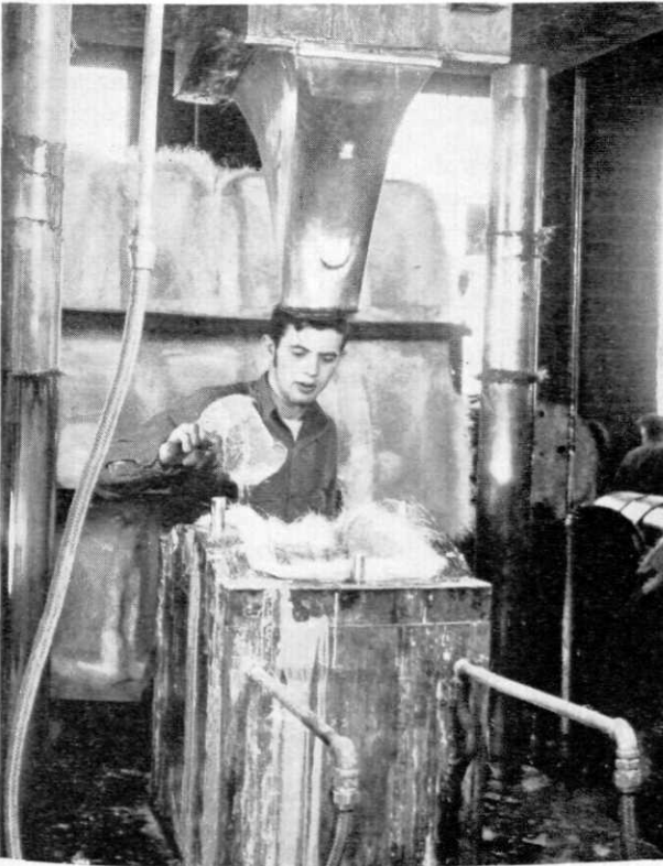
Polyester resin is poured over the preform. When the dies are closed, pressure forces the resin throughout the preform, bonding the fiberglass in a cured plastic solid.
