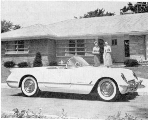
The Chevrolet Corvette—first mass-produced American sports car—features a body molded of fiberglass reinforced plastic. The Corvette, the Kaiser Darrin, and other sports cars are the most recent and most dramatic use of this material, and point toward new horizons in the automobile industry.
