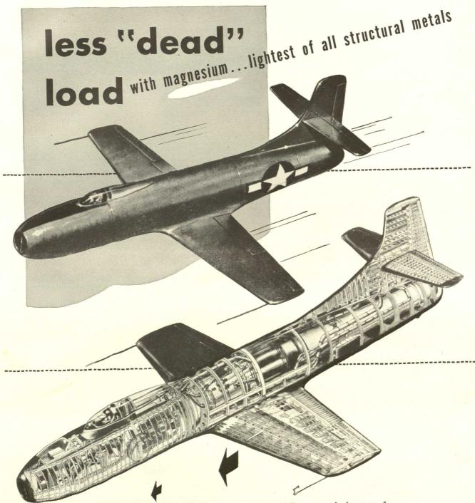
Here you see the Navy-Douglas D558 Skystreak—a dramatic demonstration of the structural advantage of magnesium. Strong magnesium alloy sheet is literally "wrapped" around the Skystreak's powerful jet engine to form the entire fuselage skin aft of the pilot seat. This makes possible a monocoque structure which completely eliminates the usual stringers, except for frames carrying concentrated loads.
