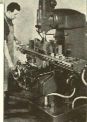
On the job shown above the work is quickly positioned for cutting several adjacent surfaces.
