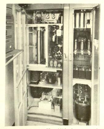
Rear view of the power amplifier and high voltage power supply. The final tank circuit with tubes in place can be seen in the enclosed box at the left. The unit on the left is the high voltage power supply.
