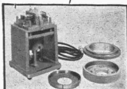
Special fixture utilizes Gage Head Cartridge and Amplifier to measure internal angle accuracy to \pm 1\frac{1}{2} seconds.
