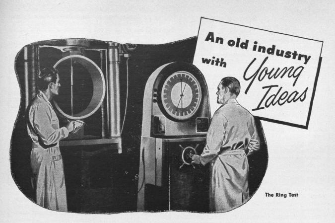
The ring test, shown above, is a scientific method for determining the modulus of rupture of pipe. It is not a required acceptance test but one of the additional tests made by cast iron pipe manufacturers to ensure that the quality of the pipe meets or exceeds standard specifications.
