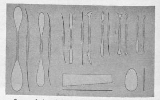
Some of the plasterer's tools include spatulas, scrapers, cutting and filing equipment, carving tools. (U. S. Gypsum Co.)
