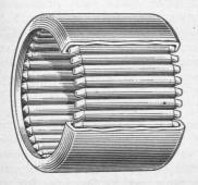
The Torrington Needle Bearing is a completely self-contained unit consisting of a full complement of small diameter rollers and a single retaining shell. This unit design and construction greatly simplify handling and speed assembly, and help reduce the size and weight of related parts.
