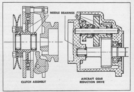
Typical installations of Torrington Needle Bearings are characterized by simplicity of design. Needle Bearings are made for shafts as small as 5/32'' up to those as large as  $7\frac{1}{4''}$ .
