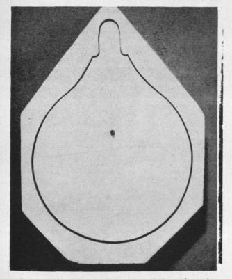
An original pattern and the expanded mold, made of high expansion cement. The neck shows that expansion is proportional. (U. S. Gypsum Co.)
