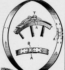
\$10.00 buys a complete set (including the tightener T) of STEEL TIRES 4½, that can be put onto the wheels of any farm wagon over the narrow tire, and can be attached or detached by one man in twenty minutes. In ordering give diameter of wheels. Address
