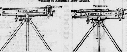
Grade Bar. B—The Level. C—Registering Scale. D—Thumb Screw to Level. E—Thumb Screw to Grade Bar. F—Back Sight. G—Globe Sight. H—Pointer on Scale. See Fig. 2.
