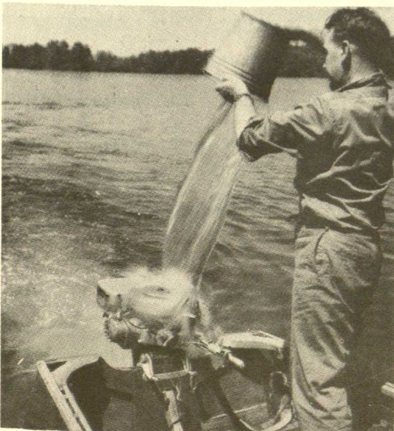
DC4 compound, developed during the war for sealing ignition systems of aircraft engines, finds many peacetime uses.
