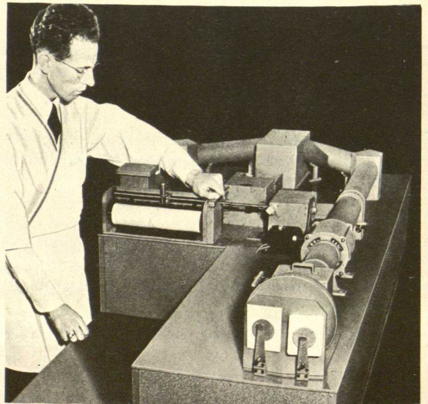
This recording spectrophotometer can detect and record more than two million different colors. (GE photo)
