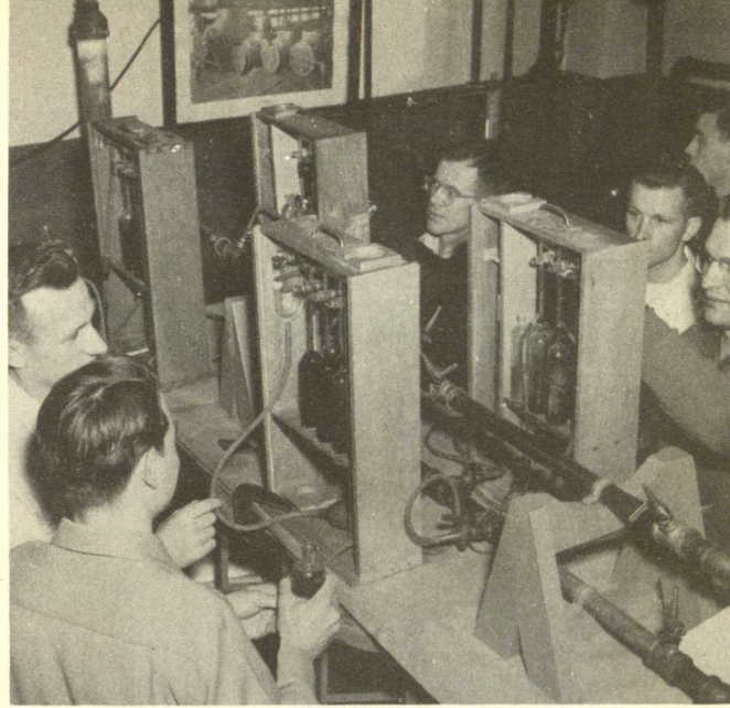
Hard at work on the Orsat test in the ME power lab.
