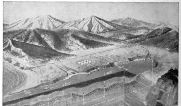
Harbor Excavation. Harbor: 4-200 KT at 800 ft. DOB. Area ~ 180 acres. Channel \geq 5 - 50 KT at 500 ft. DOB minimum depth — 50 ft. MLW.
