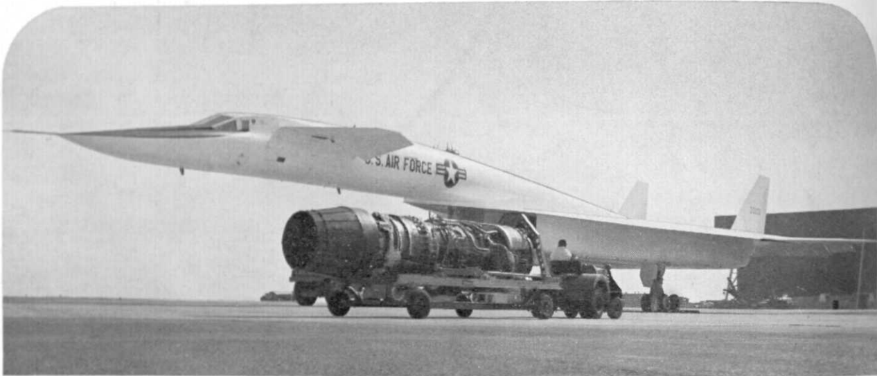
DEFENSE —G-E engineers designed and produced six J93 engines to push USAF XB-70 to Mach 3.
