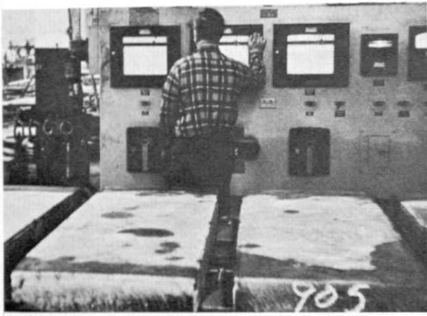
Explosion-bonded clads await furnace-softening prior to hot-rolling.
