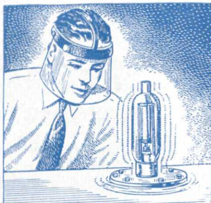
Will vibration harm tubes for aircraft radio? G-E engineers developed equipment to shake them 25 times a second for 100 hrs.
