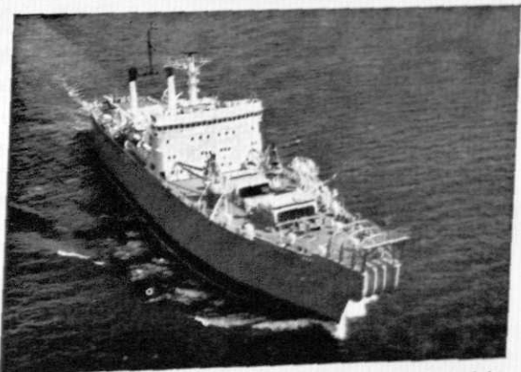
C. S. LONG LINES lays and maintains Bell System undersea telephone cables that provide dependable overseas transmission.
