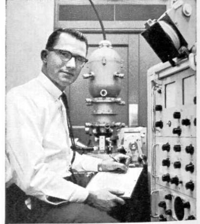
DENNIS WITMER, CH.E., MARYLAND '61 —An engineer at our research laboratories in Bethlehem, Pa., Dennis is shown using a microprobe to study corrosion-resistant coatings on sheet steel.
