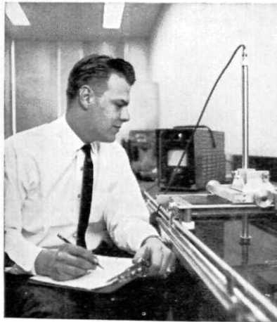
WALT BANTZ, E.E., SCRANTON '63 —Engineer at our research laboratories in Bethlehem, Pa., Walt is shown evaluating performance of ultrasonic equipment for detection of flaws in steel plates.
