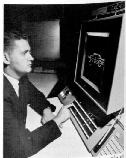
A computer programmer takes the role of an "automotive designer" to test out the new GM DAC-I system. The console can be used to monitor and control the computer's progress on a design problem. At any design stage the designer may request a permanent photographic copy of a new drawing using the special image processor.
