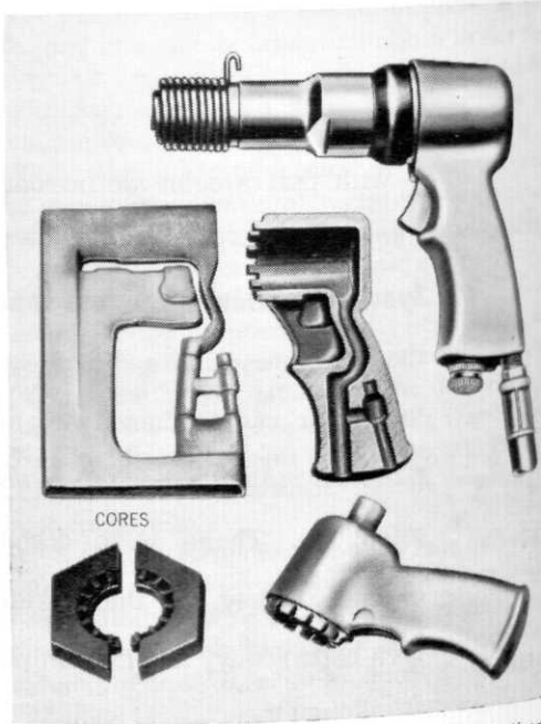
Precise dove-tails, intricate air channels and other interior details of this impact wrench handle are produced in the Malleable casting by the three shell cores shown. A variety of machining operations is eliminated by this relatively low-cost technique.
