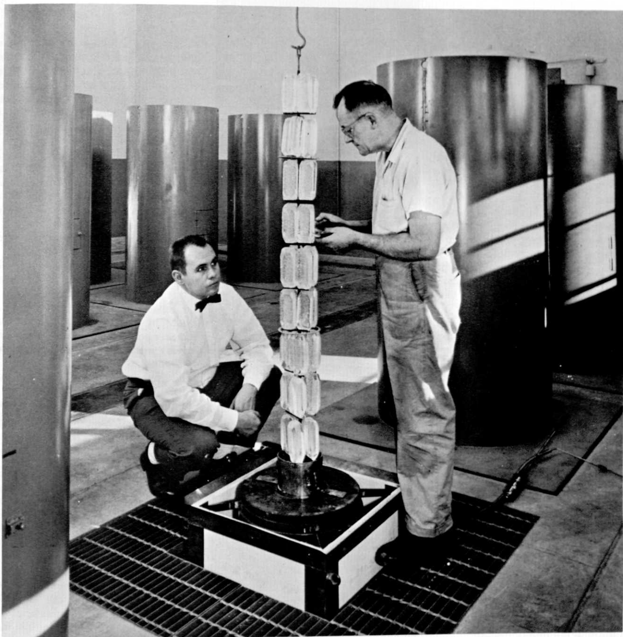
Synthetic crystals are inspected as they emerge from the growing vessel three weeks after they started growing.
