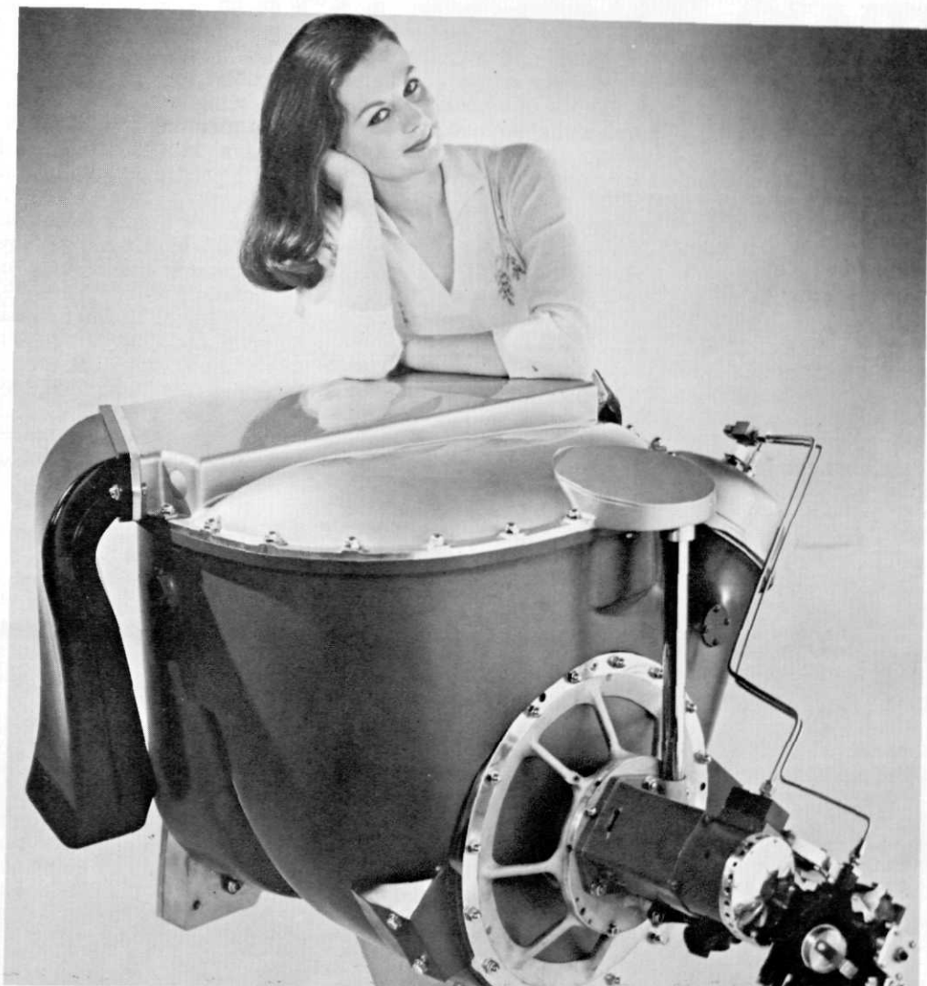
This is the gas turbine engine which, sans la mademoiselle, powered a 1962 Dodge Turbo Dart on a test run from New York to Los Angeles.
