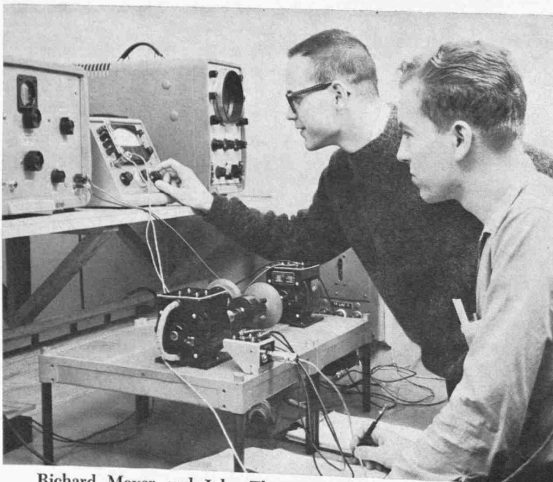
Richard Meyer and John Thornton measure the terminal characteristics of a D.C. machine.
