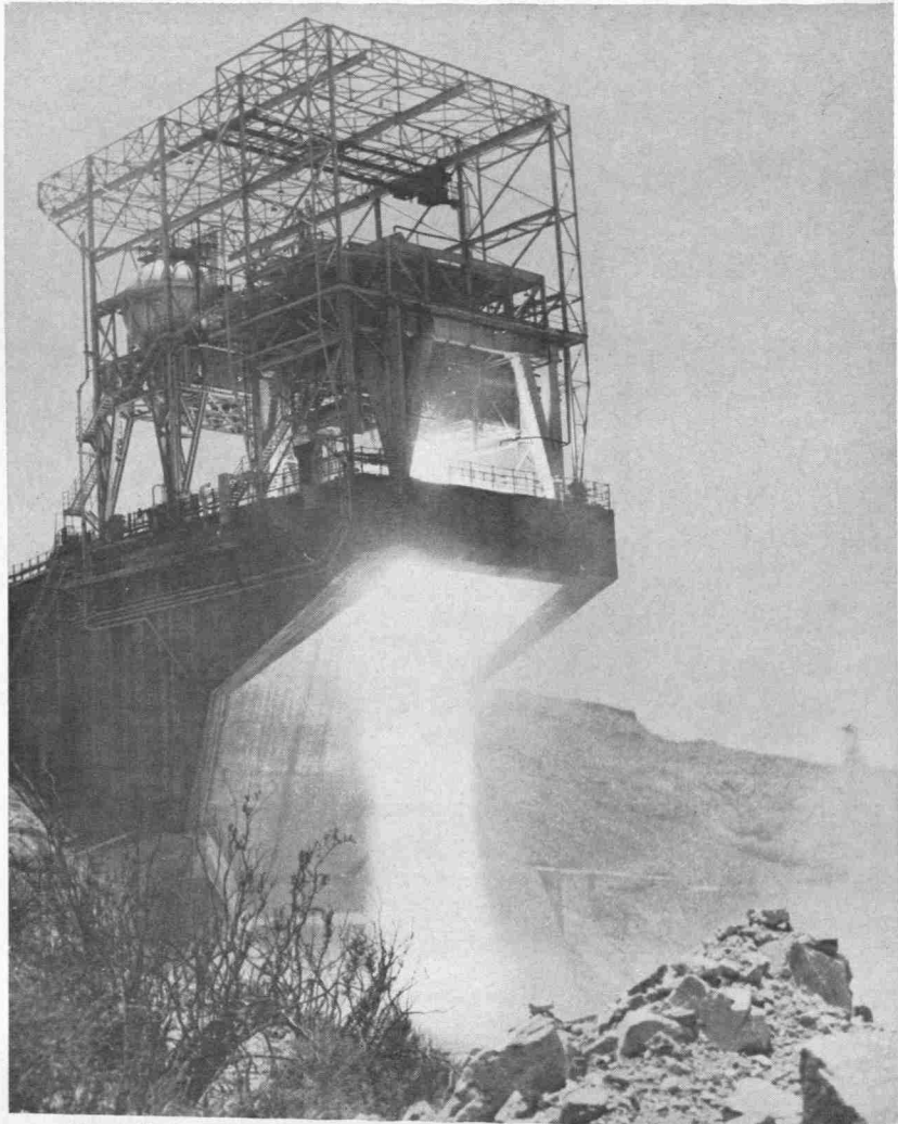
More than one million pounds of thrust streams from F-1 rocket engine during first series of tests of a complete flyable system. The F-1 is the free world's most powerful space booster engine.
