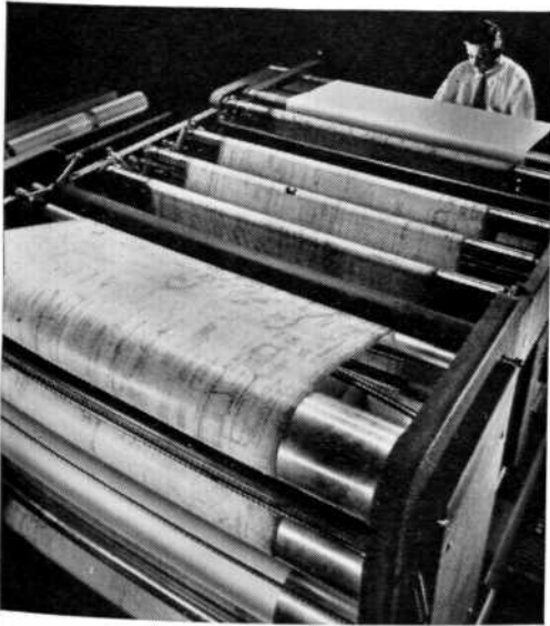
Giant machines produce a flow of photo-exact engineering drawings—save countless hours of drafting time.
