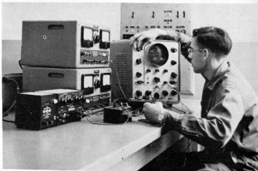
Mr. B. Rose determining the square wave characteristics of a laboratory amplifier.
