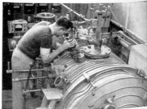
Vacuum melting has opened up new horizons for development of alloys. Here, a Pratt & Whitney Aircraft metallurgist is shown as he supervises preparation of an experimental high-strength nickel-base alloy, melted and cast under high vacuum.
