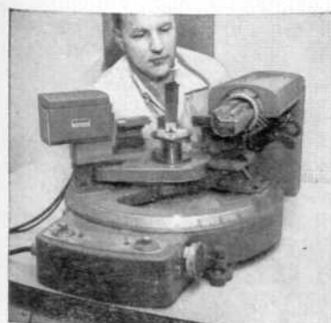
Engineer measures residual stress in a compressor blade non-destructively, using X-ray diffraction. Stress analysis plays important part in developing advanced aircraft engine designs.
