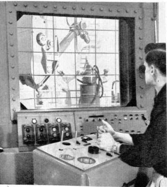
GIANT HAND —A technician operates a huge mechanical "hand" at AEC's aircraft nuclear propulsion test site, Idaho Falls, Ida. Designed and built by General Electric, the manipulator can handle from 500 to 3,000 pounds and can easily disassemble an aircraft jet engine, bolt by bolt.
