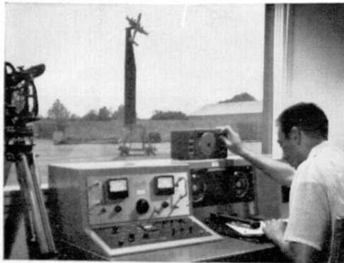
Electronics Research Engineer Irving Alne records radiation antenna pattern on Lockheed's Radar Range. Twenty-two foot plastic tower in background minimizes ground reflections, approximates free space. Pattern integrator, high gain amplifier, square root amplifier and logarithmic amplifier shown in picture are of Lockheed design.
