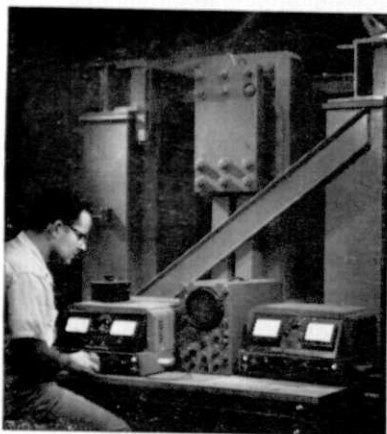
Research Engineer Russell Lowe measures dynamic strain applied by Lockheed's 500,000 lb. Force Fatigue Machine on test specimen of integrally-stiffened Super Constellation skin. The Fatigue Machine gives Structures Department engineers a significant advantage in simulating effect of flight loads on a structure. Among other Lockheed structures facilities are the only shimmy tower in private industry and largest drop test tower in the nation.
