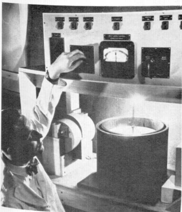
A scientist raises the level of molten titanium in a gamma ray controlled purifying furnace.
