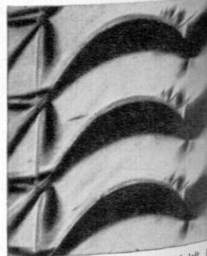
Schlieren photographs, above and left, illustrate different phases of airflow investigation. Development of inlets, compressors and turbines requires many such studies in cascade test rigs, subsonic or supersonic wind tunnels.
