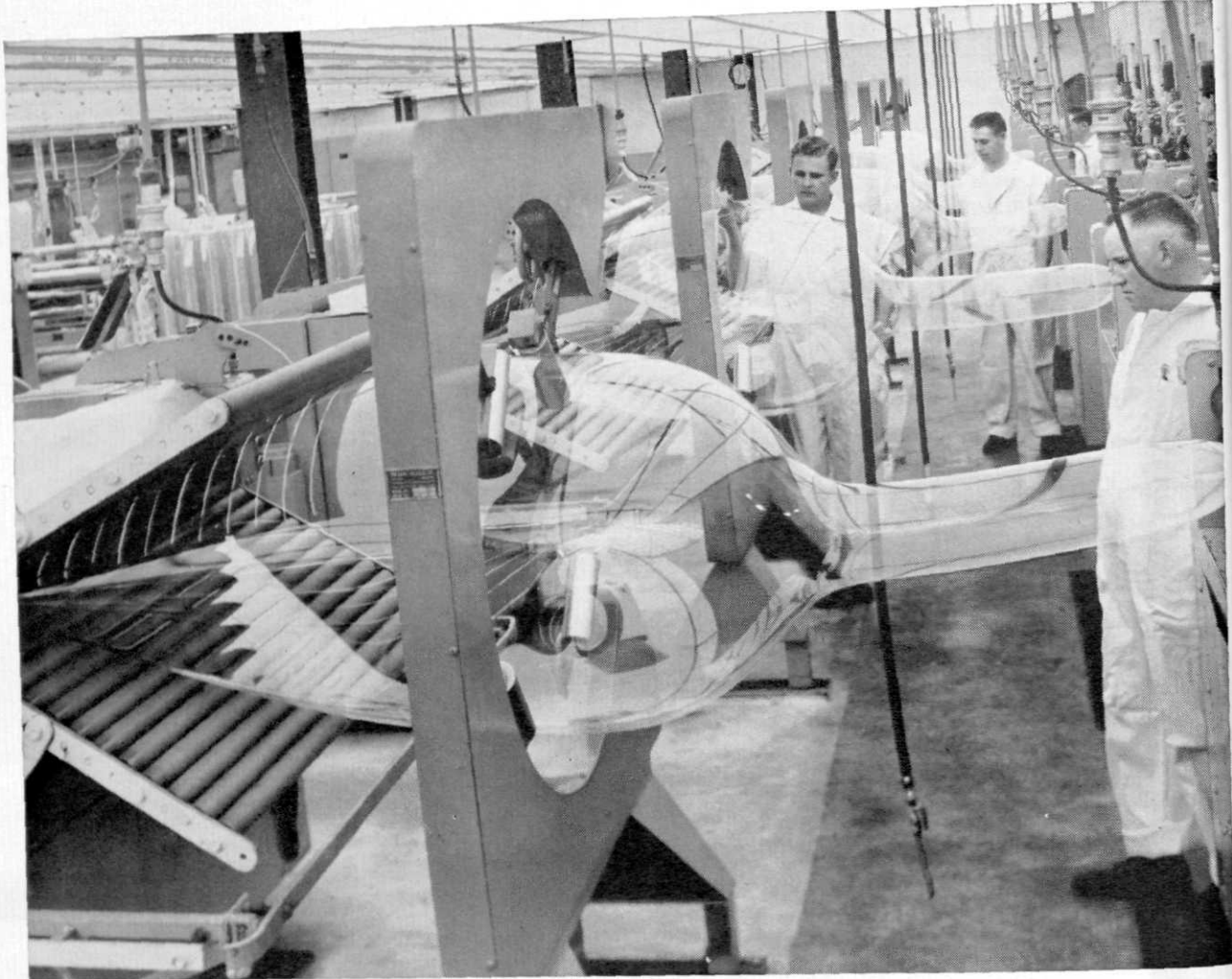
Saran Wrap is stretched by injecting compressed air to form a bubble \frac{1}{2} mil in thickness which is then compressed and wound.
