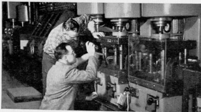
Here Dick and a set-up man check over the automatic production line used to manufacture a wire spring relay part for complex telephone switching equipment. This automatic line carries a component of the relay on a reciprocating conveyor through as many as nine different and very precise operations—such as percussive welding in which small block contacts of palladium are attached to the tips of wires to within a tolerance of \pm .002 ".
