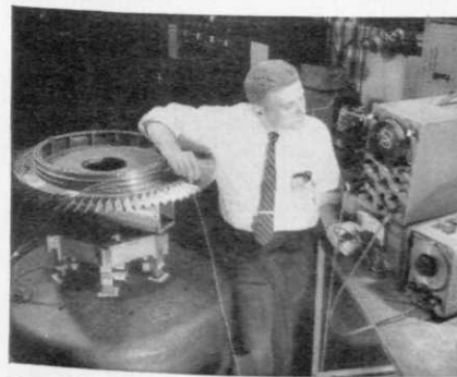
Instrumentation engineer at Pratt & Whitney Aircraft is shown investigating modes of vibration in a blade of a single stage of a jet engine compressor.
