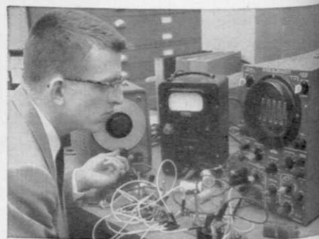
Pratt & Whitney Aircraft engineer checks a bread board model for a subminiature, encapsulated amplifier built with transistors.
