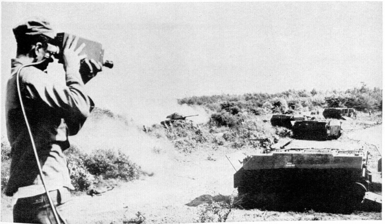
Vidicon camera, carried in armored amphibious personnel carrier, is shown in operation at demonstration. Picture of actual landing from the amphibious vehicle was micro-waved several miles to "command post of the future" where regimental officers were able to evaluate the progress of the "assault."
