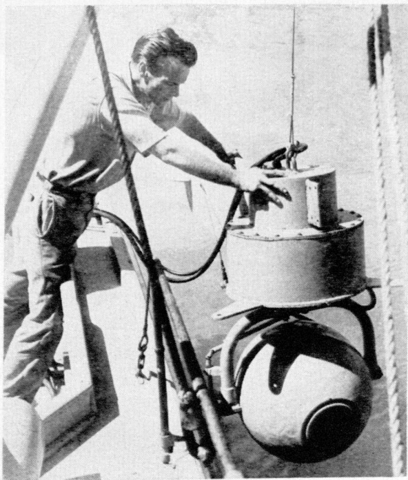
Underwater application of closed-circuit television is enabling U.S. Fish and Wildlife Service to remotely observe and test performance of experimental fishery methods and equipment under actual oceanic conditions.
