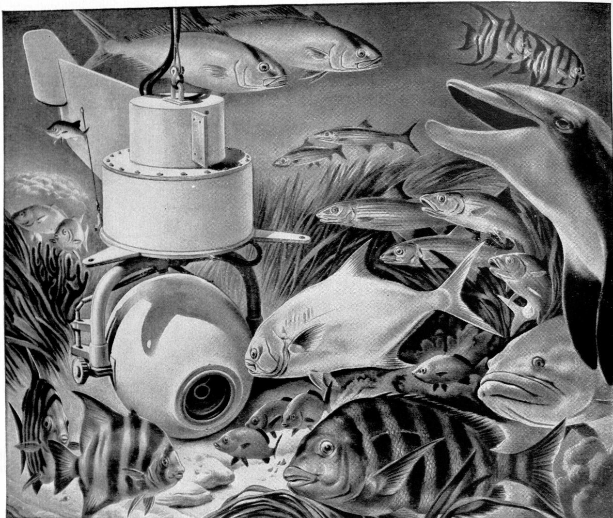
RCA TV camera encased in special diving bell televises the activities of sea life in sunlit waters off the Gulf Stream.
