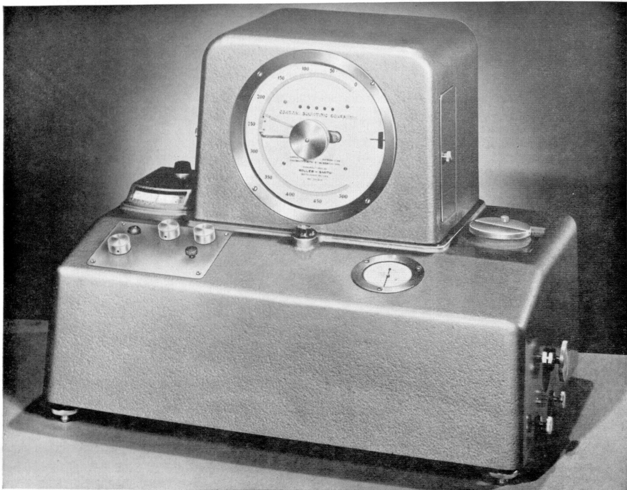
THE PERCENTAGE of hydrogen in liquid hydrocarbons can be determined by making two simultaneous measurements on the sample to give (1) density and (2) the absorption rate for beta rays. The weight percentage of hydro-
