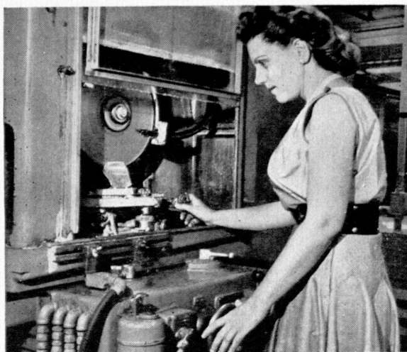
Quartz stones are cut into wafers on this diamond-edged saw, with orientation to optical axis controlled by fixture. This is just one of several types of machines designed and developed by Western Electric engineers to mechanize quartz cutting.
