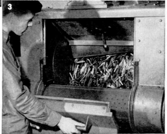
TUMBLING — Prior to inspection and packaging, REX High Speed Tool Bits are cleaned by tumbling.
