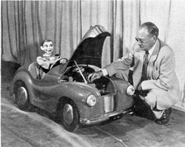
Zworykin Inspects Electrically Controlled Auto. Dr. V. K. Zworykin, pioneer electronic scientist, examines electronic apparatus of model car that drives itself. The car has been equipped in a study of problems of avoiding accidents and of automatic driving on super-highways of the future. The experimental car keeps itself centered over the wire, which radiates a signal. It can automatically stop or turn into another lane when another car is in its path.
