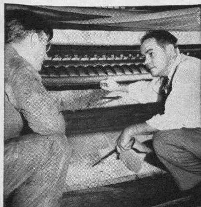
Edgar G. Boyce, Ashland State (right), helps a customer improve his method of applying silicate adhesive in the manufacture of corrugated boxboard.
