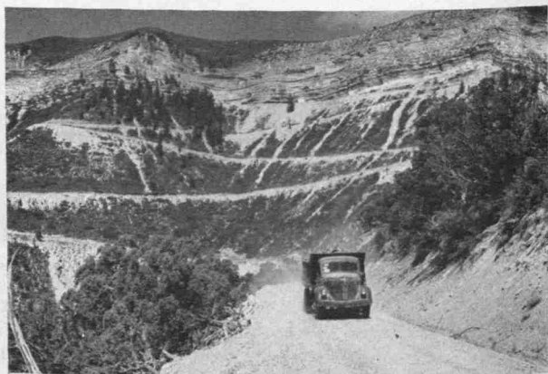
Oil shale is quarried rather than mined, for the cost of removing the ore by mining techniques would be prohibitive. Under ground electric shovels dump the ore directly into Diesel trucks for removal from the underground quarry.
