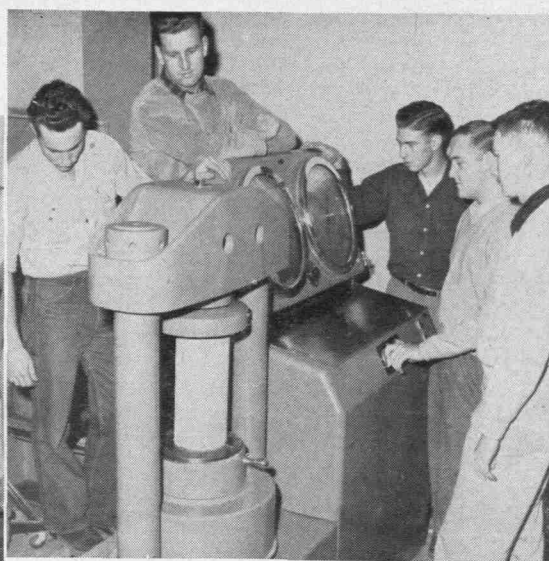
Breaking a concrete test specimen in the C.E. Lab.
