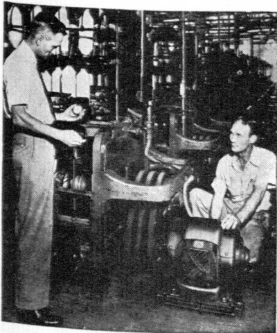
Textile mills are getting adjustable speed at lower cost by using new automatic Vari-Pitch sheaves on spinning frames as shown.
