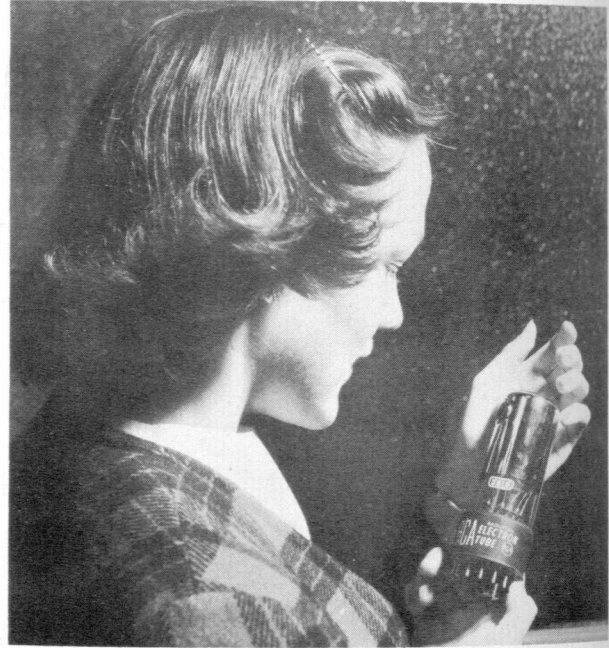
A Multiplier Phototube which is used in the Scintillation Counter.
