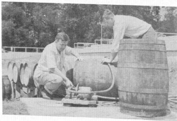
Pumping the pickling liquor waste from the supply source to the aerators.
