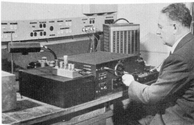
The phototube of this experimental scintillation counter is in the black tube at the left. The instrument at the right analyzes and counts the electric impulses.
