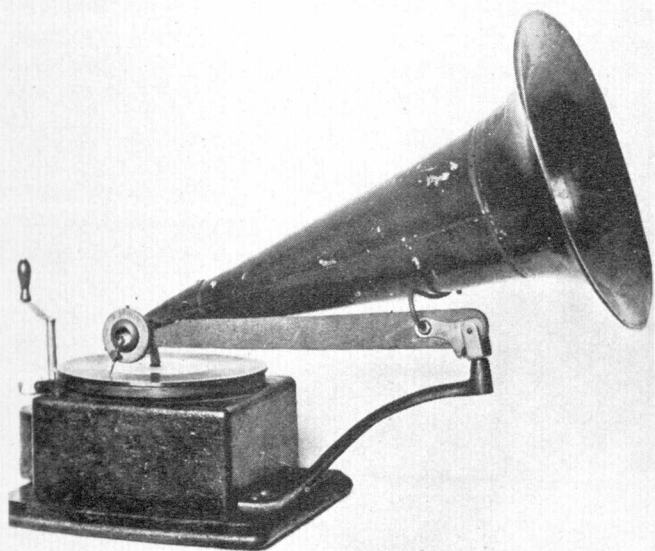
The Berliner Gramophone, patented in 1887, featured a flat disc and a horn, in contrast to the cylindrical records then in common use.
